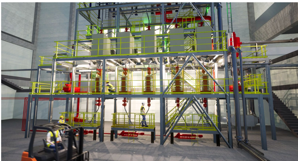
Figure 1 – Front end section of Silumina Plant design
